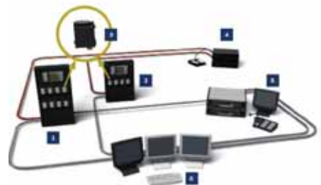
Data interface to Plena Public Address and Voice Alarm System
